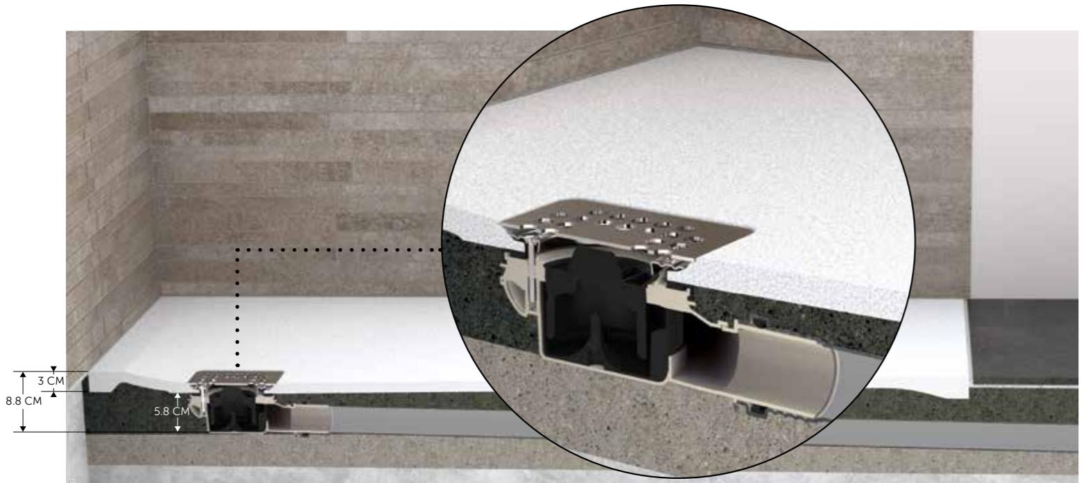
RAK-Feeling shower trays can be installed flush to floor, semi-recessed or directly onto the floor.. RAK-Feeling products are ideal for both new buildings and renovations, thanks to the minimum dimensions of 5.8 cm required under the shower tray for the waste.
