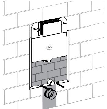
The concealed cistern can be easily fastened in front of or inside a solid wall and then brick lined.
