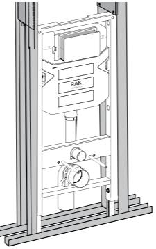
With a drywall system it is possible to create complete room-height prewalls or partitions.
