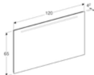
120cm mirror with functional lighting from the top W 120 / D 4.2 / H 65cm Mechanical switch, LED lighting. Art. no. 500.585.00.1
