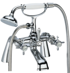
Bath Shower Mixer & Handset Min recommended pressure 0.1bar 235(w) x 270(h) x 200(d)mm
