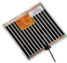
Mirror Heater Pad 230V - 200 W/m2 IP Rating 44 Power Rating 50W Copper with Carbon Connections 1mm Thickness 500 x 530 mm
