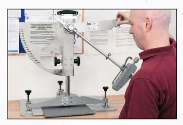
This test is designed to simulate the action of a slipping foot and uses a weighted swinging arm which contacts the surface of the tile with a standard rubber slider that represents the rubber sole of a shoe in both dry and wet conditions. The slip resistance is the upswing measured from a scale on the instrument. The greater the upswing, the lower the slip resistance and the greater the slip potential.
