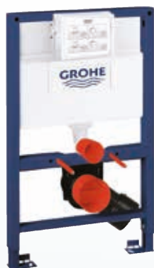
Rapid SL WC. 820mm height Dual flush cistern, 3L/6L front or top actuation requires front wall fixing brackets 3855800M . Requires wall plate actuation or remote pneumatic actuation 37060 , 37059
