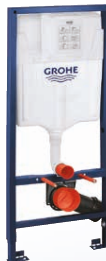
Rapid SL WC. 1130mm height Dual flush or start/stop actuation cistern, 2.6L/6L front actuation Requires front wall fixing brackets 3855800M requires wall plate actuation
